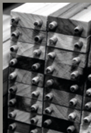
Stronger build process using double dowels and glue.
